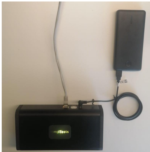
Figure 5: Ethernet and power bank connections
