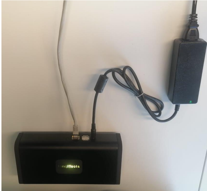
Figure 6: Ethernet and mains power supply connections
